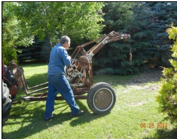
Carl demonstrating hand cranking the 1920s Manley Wrecking Crane tow truck boom crane. The Vanden Heuvels used this machine to move and position all 800 tons of stone in their yard. They attached chains around each stone, lifted it with the ‘Wrecker’, then moved the stone (using the 1972 IH tractor attached to the Wrecker (on left) into position. Some of the stones exceeded three tons each.
